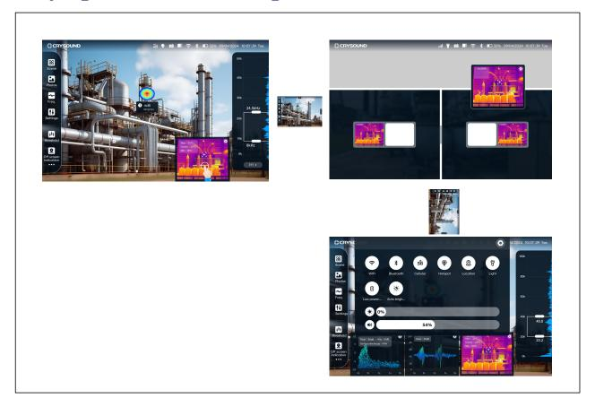
Long pressing the thermal image enters the dragging mode, allowing you to drag the thermal image to the upper area of the main screen to display it in the thermal view. Dragging the thermal image to the left or right area enters the split-screen display mode.
